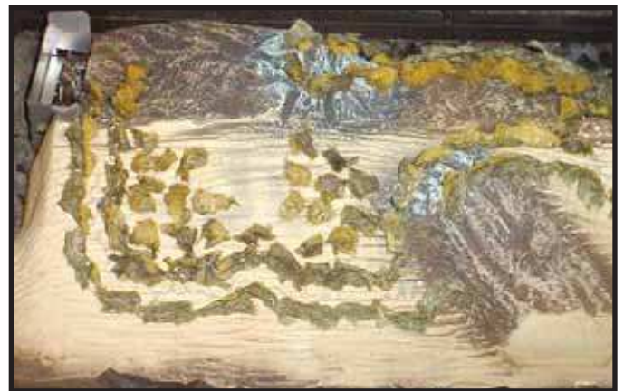
Figure 11.2 Placement of Ember Materials
