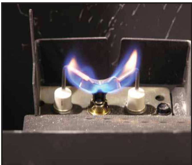
Figure 3.1 IPI Pilot Flame Pattern
