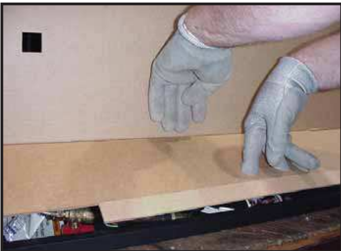
Figure 13.12 Opening Lower Access Panel
