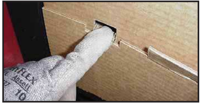
Figure 13.13 Securing Tabs Inside Front of Splatter Guard
