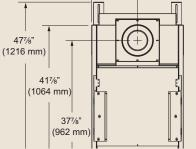
Framing dimensions in illustrations accommodate 1/2" finishing material.
