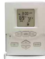
Programmable wireless wall thermostat with receiver
