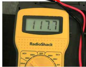
Should read between 110 and 120 volts ac.
