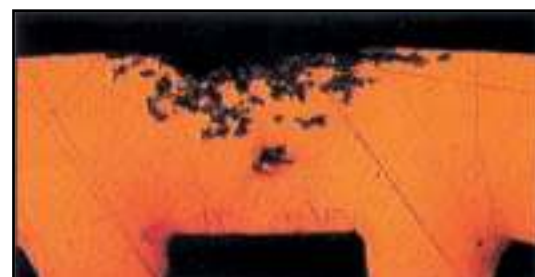
Fig. 2 Formicary Corrosion Tunneling
