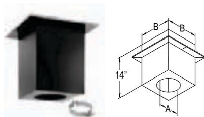
Use to pass through ceiling and support pipe. May be used on vaulted or flat ceilings. Painted black. Trim and clamp included.
