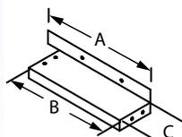
Use as a heat shield on structures with vinyl siding, or other temperature sensitive materials, to help prevent warping and or melting of the material. Use only on horizontal terminations and on any irregular surfaced siding (ie: ship lag siding, shake shingle siding) so cap is not imbedded in the siding. Kit includes 4-pieces; sized for Sconce Cap and Round Horizontal Cap only. Stainless steel (SS) and Copper (C) available. Use for 4" x 6 5/8" and 5" x 8" diameters.
