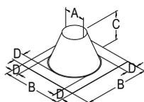
Use to weather proof the penetration of vent pipe through the roof. Storm Collar required. Use on flat roofs, chase enclosures, or masonry chimney. Made of galvalume.
