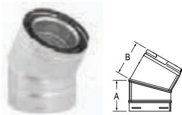
Use to offset obstructions as needed. Fully unitized, twist-lock construction. Elbows swivel, allowing the lock to remain fully engaged while aligning to the desired direction. The angle will remain fixed at 30°.
