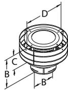
Use for vertical terminations only. Check the appliance manufacturer's instructions to determine which caps are approved for use with their appliance. Available in aluminum and stainless steel (S).
