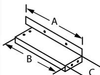
Use as a heat shield on structures with vinyl siding, or other temperature sensitive materials, to help prevent warping and or melting of the material. Use only on horizontal terminations and on any irregular surfaced siding (ie: ship lag siding, shake shingle siding) so cap is not imbedded in the siding. Kit includes 4-pieces; sized for Square Horizontal Cap only. Stainless steel (SS) and Copper (C) available.
