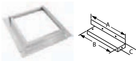
Prevents water intrusion into stucco-sided homes. Allows the installer to apply siding material (ie: stucco, brick, etc) over the flanges up to the sides of the flashing for a water-tight seal. Kit includes 4-pieces; sized for 4" x 6 5/8" Sconce Cap and Round Horizontal Cap only. Also available in stainless steel (S). Use for 4"x 6 5/8" and 5"x 8" diameters.
