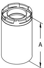
Use to add length to a straight length of DirectVent Pro. 8 1/2" pipe adds 3"- 7" of length, 16" pipe adds 3"- 14 1/2" of length, when used with rigid sections of pipe. Direct vent lengths feature a fully unitized, twist-lock construction. Use of sealant is optional, unless specified by the appliance manufacturer. Available in black or galvalume exterior (both feature laser-welded outer wall seams). Does not fit DirectVent GS pipe.
