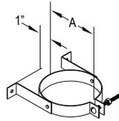
Use to support vent pipe. Provides 1" clearance. Recommend installing Wall Straps at 4-foot intervals on vertical runs.
