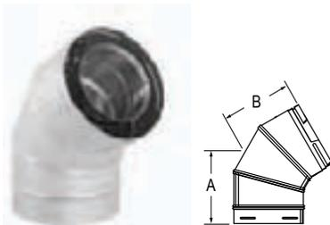
Use to offset obstructions as needed. Fully unitized, twist-lock construction. Elbows swivel, allowing the lock to remain fully engaged while aligning to the desired direction. The angle will remain fixed at 60°.
