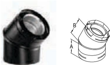
Use to offset obstructions as needed. Fully unitized, twist-lock construction. Elbows swivel, allowing the lock to remain fully engaged while aligning to the desired direction. The angle will remain fixed at 45°.
