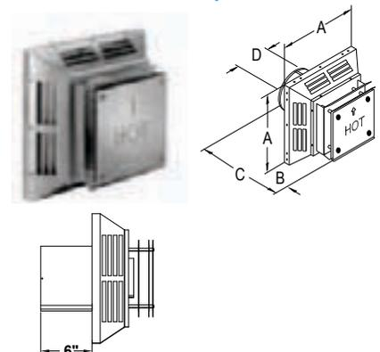
Use for standard and high-wind through-the-wall terminations. Check installation instructions for restrictions on horizontal cap terminations, such as minimum distance from windows and doors. Available in aluminum, stainless steel (S), and copper (C).
