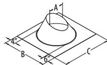
Use to weather proof the penetration of vent pipe through the roof. Storm Collar required. Select roof flashing based on pitch of roof. For pitches of 0/12 - 6/12. Made of galvalume.
