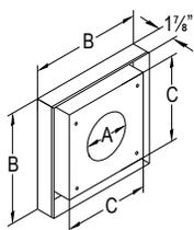
Use as a heat shield on structures with vinyl siding, or other temperature sensitive materials, to help prevent warping and or melting of the material. Use only on horizontal terminations and on any irregular surfaced siding (ie: ship lap siding, shake shingle siding) so cap is not imbedded in the siding. Sized for Square Horizontal Cap.
