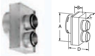
Use Co-Linear Adapter for stoves with 4" X 6 5/8" co-axial outlets. Refer to appliance manufacturer's installation instructions for approval. Uses 3" aluminum flex for both intake and exhaust.
