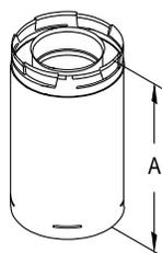
Designed for appliances tested and listed for direct vent. Features a fully unitized twist-lock construction in both 4" x 6 5/8" and 5" x 8" vent sizes. Use of sealant is optional, unless specified by the appliance manufacturer. To calculate install length, subtract 1 1/2" for each joint. No beads or hems. Black pipe lengths feature exterior laser-welded seams.
