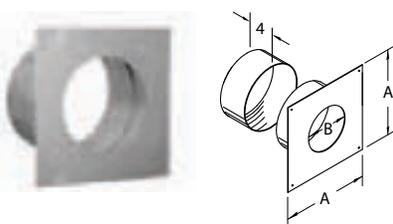
Provides a complete wall-pass-through and interior firestop. Features an adjustable sleeve for an exact fit. Eliminates visible trim on exterior or wall near cap. Sized to fit all DuraVent Direct-Vent Pro's termination caps.
