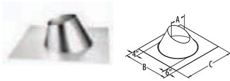
Use with metal or tile roofs. Available in sizes 4" x 6 5/8" and 5" x 8", in 0/12-6/12 (shown) and 7/12-12/12 styles. Made of malleable dead soft aluminum. Refer to roof flashings tables (previous page) for dimensions.
