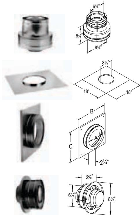
Kit 46DVA-KMC includes: Cap Adapter, 18" x 18" Flashing, Round Ceiling Support/Wall Thimble Cover, Retro Connector. For 4" x 6 5/8" direct vent. Termination Cap and 4" flex are sold separately.
