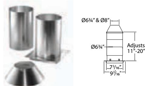
Required for installations that pass through an attic to prevent insulation and debris from accumulating near the vent. Provides 1" clearance to combustibles.
