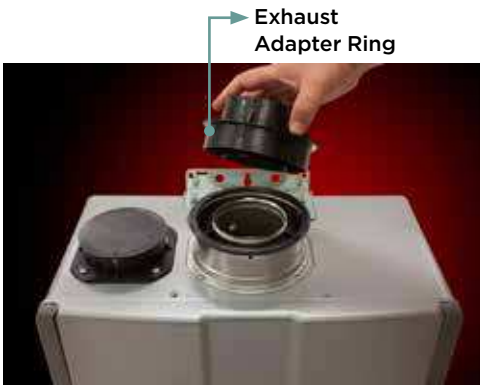
For concentric venting, installers simply remove and discard the exhaust adapter ring.
