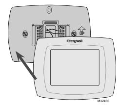
Align pins on back of thermostat with slots in wallplate, then push gently until thermostat snaps into place.
