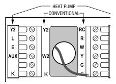
Connect the common side of the transformer to "C" terminal. This connection is mandatory.
