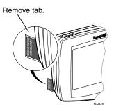
The thermostat is shipped from the factory with the coin cell installed. To keep the battery from discharging during shipment and storage, the thermostat is shipped with a plastic tab inserted in the battery holder. This tab must be removed during installation. Simply pull the plastic tab out of the battery tray. Make sure that the battery tray is fully inserted into the thermostat.
