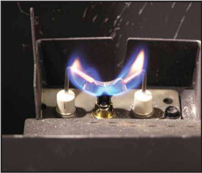
Figure 3.1 IPI Pilot Flame Pattern
