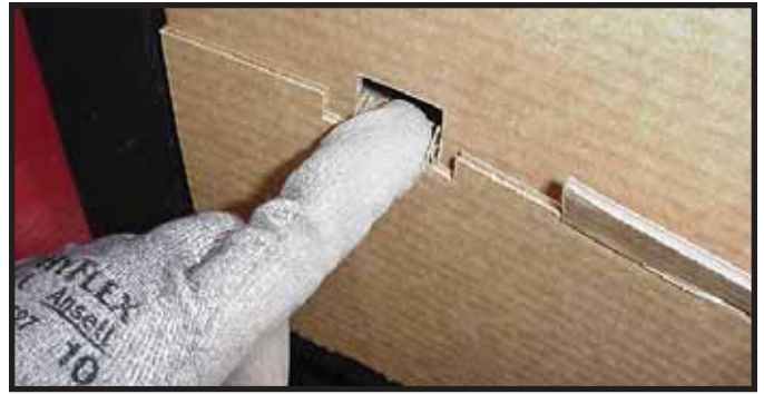
Figure 13.13 Securing Tabs Inside Front of Splatter Guard
