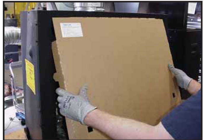
Figure 13.8 Installation of Splatter Guard
