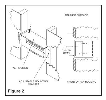
**NOTE**: If the fan housing is installed in a  $2 \times 4$  wall, the front of the housing will protrude approximately 1/2 - in. (13mm) out of the wall. See Figure 3.
