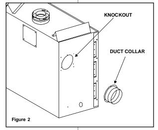
**NOTE:** The fan duct assembly may be mounted anywhere in the flex duct run that may be convenient. The fan duct collar may need to be crimped to accept the flex ducting. Take care to secure the fan against nuisance vibration. Tape all seams with aluminum tape.
