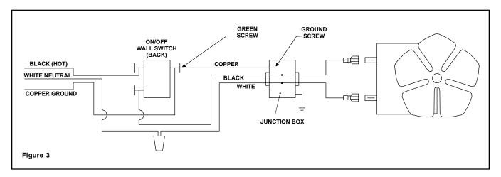
Wire the fan to the wall switch (see Figure 3). Attach the junction box to the fan duct assembly. Use the strain relief to secure the wire through the wall of the junction box.
