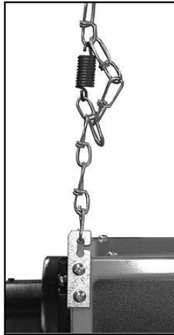
Fig. 6 - Chain Spring Installation
