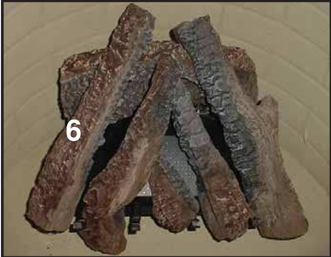
LOG #6 (SRV704-701): Place log #6 on left side of grate. Position the base of the log on the log tab. Log tab should insert into slot feature on back side of log. Place the top of the log into flat spot on log #1.
