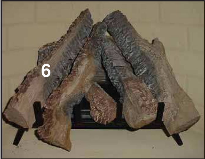
LOG #6 (SRV704-701): Place log #6 on left side of grate. Position the base of the log on the log tab. Log tab should insert into slot feature on back side of log. Place the top of the log into flat spot on log #1.
