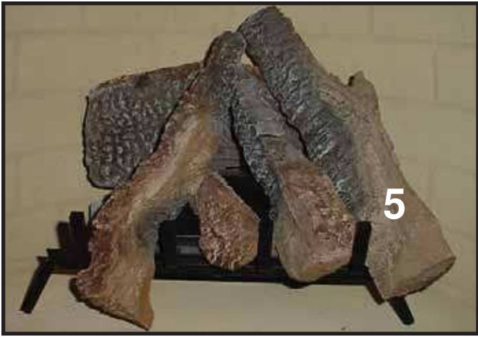
LOG #5 (SRV704-702): Place log #5 on right side of the grate. Position the base of the log on the log tab. The log tab should insert into slot feature on back side of log. Place the top of the log into the groove on log #1.
